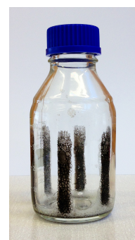
Fig 3. A 500 ml flask containing LOABeads magnetic particles, after separation and removal of liquid in the LOABeads MagSep 500 separator.
