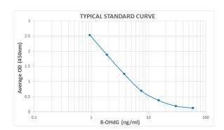
Typical Standard Curve for the DNA Damage (8-OHdG) ELISA kit (Enzyme-Linked Immunosorbent Assay) StressXpress® – SKT-120. Assay Type: Competitive ELISA. Detection Method: Colorimetric Assay. Assay Range: 0.94 – 60 ng/ml.
